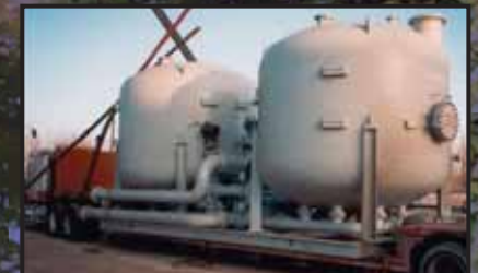
GRANULAR ACTIVATED CARBON VESSELS BEING DELIVERED TO A SITE
